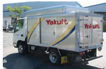
Route delivery truck with a container collection space attached to the roof
