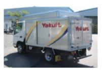
Route delivery truck with a container collection space attached to the roof
