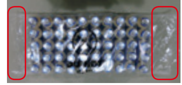
Transparent shrink-wrap film. The size of both ends was reduced to save plastic.
