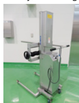
Aluminum foil transportation trolley introduced to reduce workload
